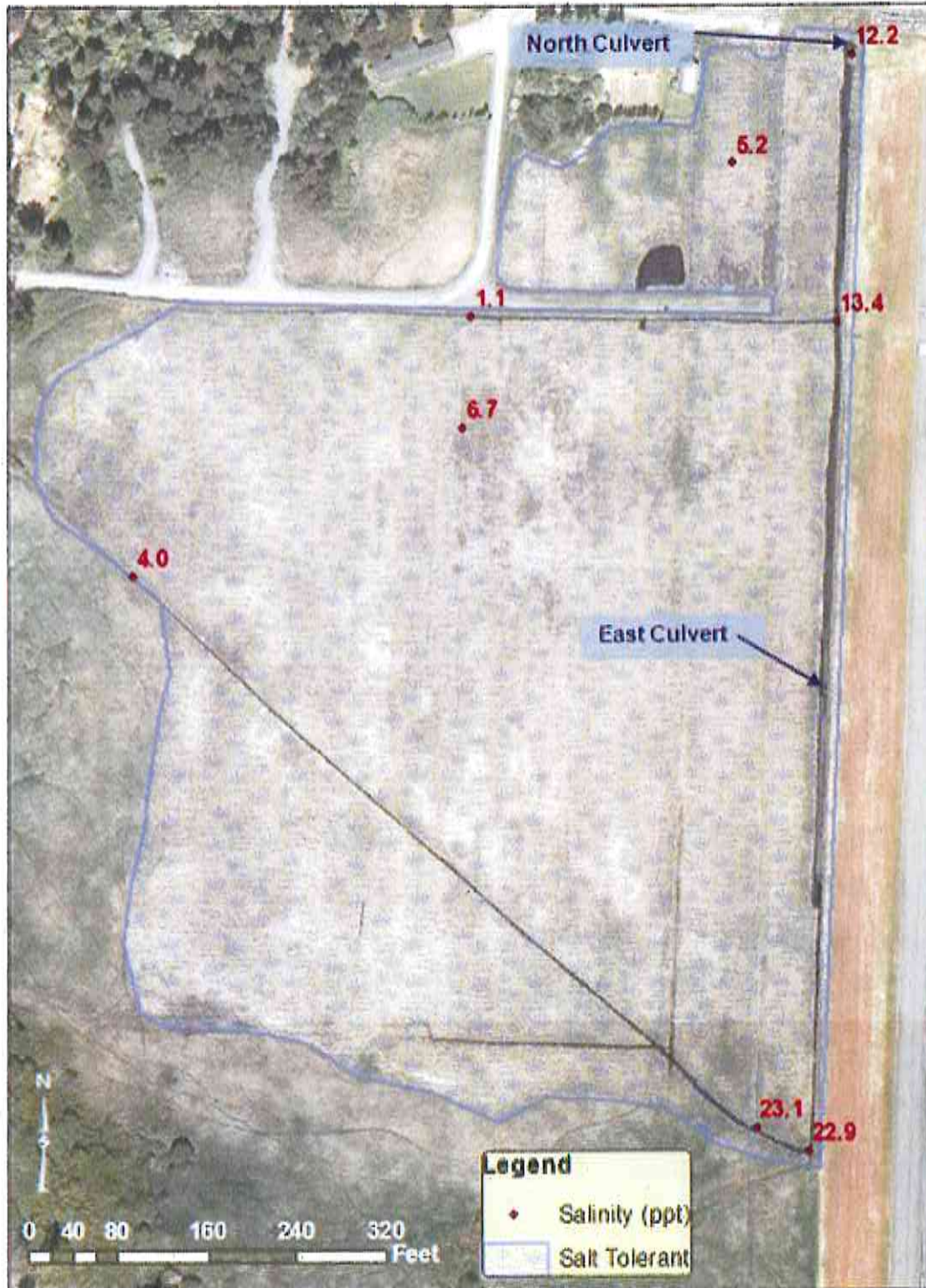
Figure 1. Measured salinities and estimated extent of salt tolerant vegetation, Wetland B.
